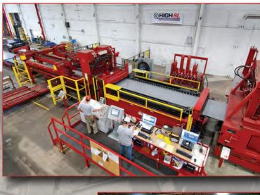
Red Bud Industries stretcher leveler technology precisely grasps the sheet or plate, up to one-half-inch thick, and stretches it past the material's yield point removing all internal stresses
